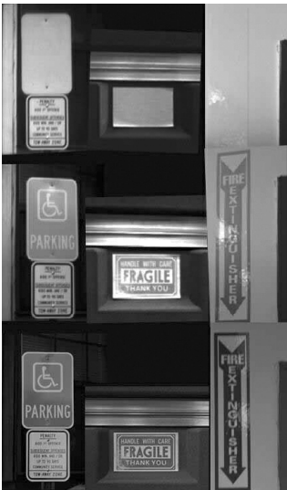
FIGURE 3. Rows of pictures are taken with an InGaAs SWIR camera (top), an InGaAs visible-SWIR camera (center), and a visible camera (bottom). Only black lettering shows up in the SWIR imagery. The blue and red lettering used in most of the warning signs can be seen with the visible-SWIR camera, but not with the SWIR-only camera.
